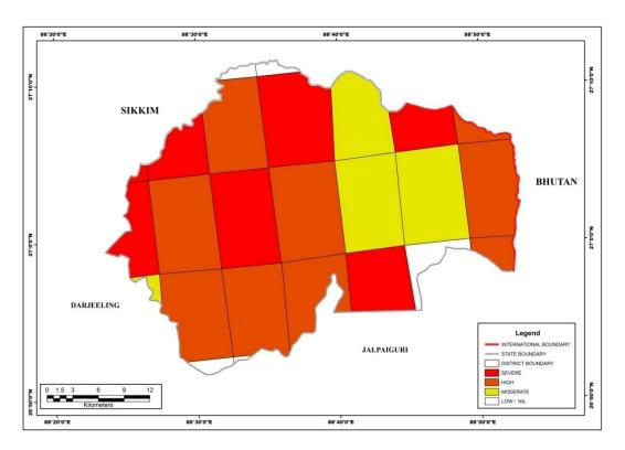
Figure 3.12: Landslide Hazard Zonation Map of Kalimpong District
